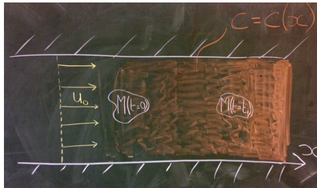
Figure 2.4: Evolution of a fluid element through a spatial gradient in concentration c = c(x) showing that the concentration inside the fluid element will change from t = 0 to t = t_1 even though the flow is steady \partial_t \mathbf{u} = \mathbf{0} .
